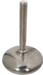
Part. R0749 - Pag. R42 Ø 120 • Stainless steel • Hygiene • Max. load 25000 N.
