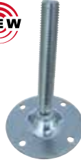
Part. R0349 - Pag. R40 Ø 123 • N. 4 holes • Stainless steel and zinc plated steel • Max. load 10000 N.
