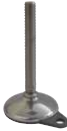
Part. R0747F - Pag. R43 Ø 80 • Stainless steel • Hygiene • Prefitting for fixing • Max. load 25000 N.
